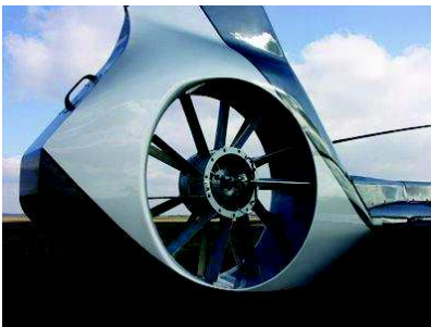
Rotor anti-couple "fenestron"
